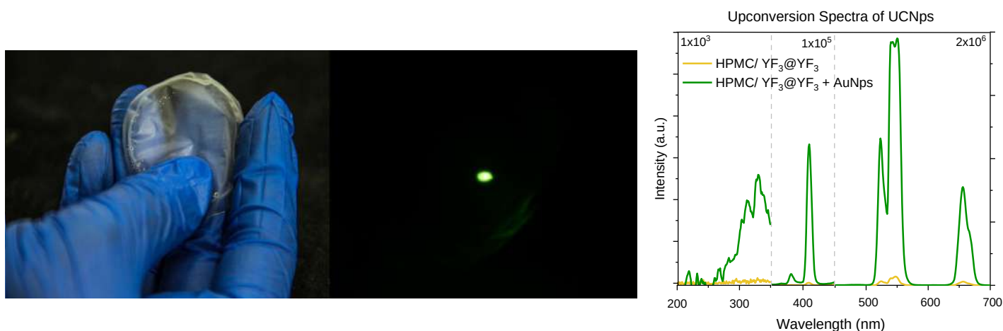
Figure 1: Photograph of the HPMC/UCNps+AuNps film in white light and with 980 nm laser excitation, and upconversion spectra of the HPMC/UCNps with added AuNps and without.
